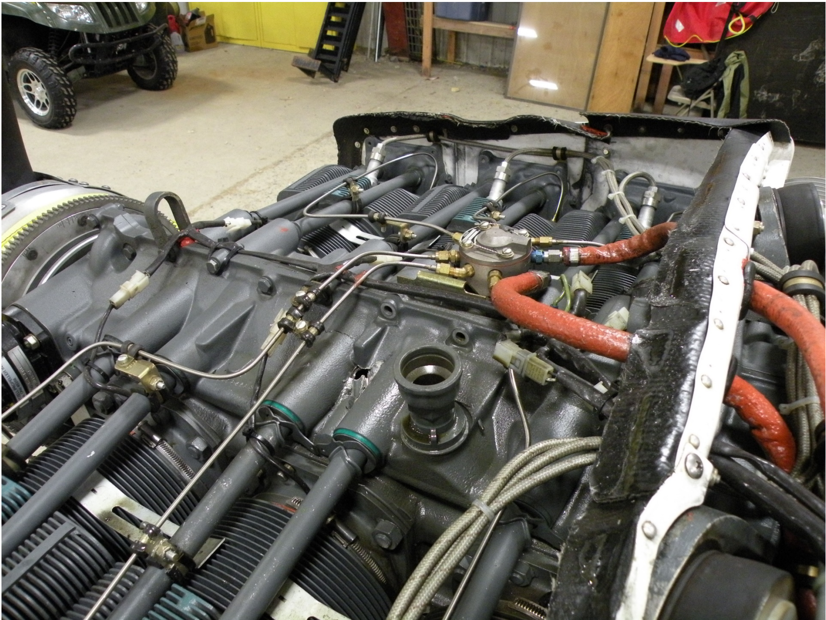
Photo 3 - Top left view of Lycoming IO-540-K1G5 exhibiting a hole and fractures at the no. 4 cylinder and a missing oil dipstick.
