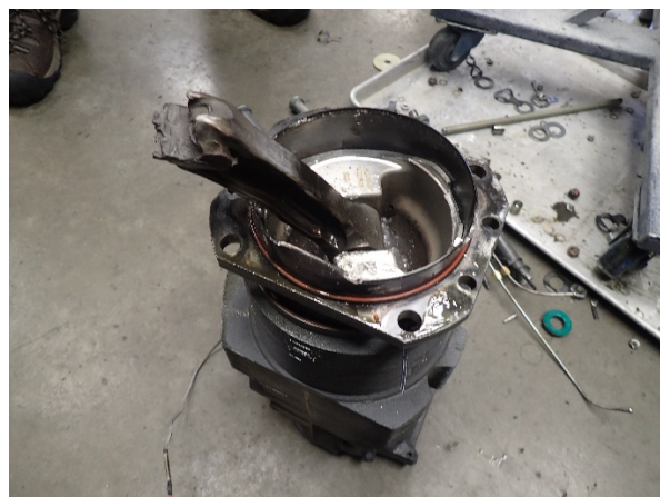
Figure 9. No. 3 and 5 connecting rod fractures and deformation (left) and no. 4 cylinder, piston and damaged connecting rod (right)
