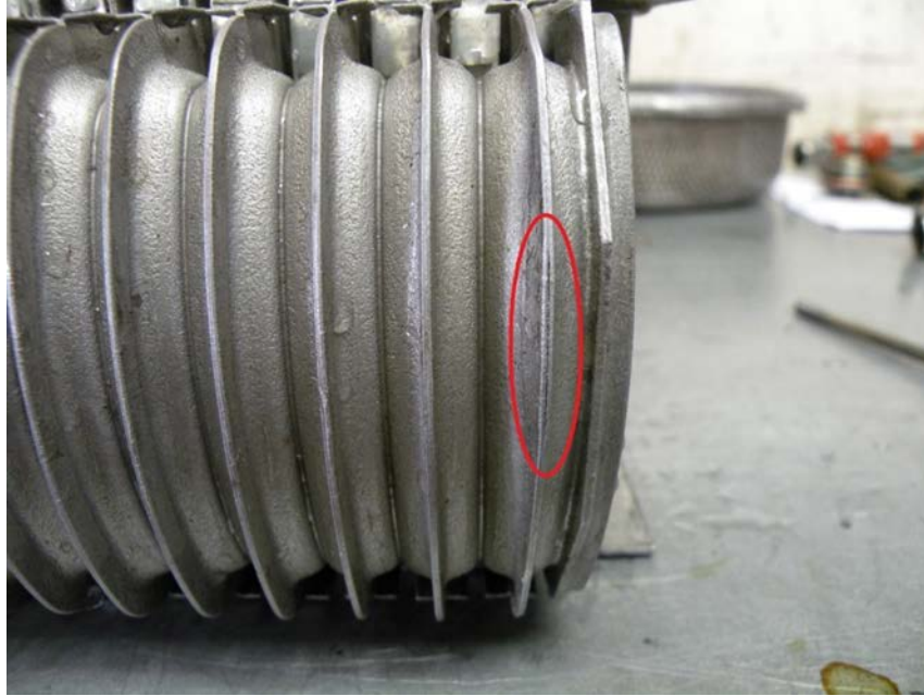
Figure 8. Aero-Classic oil cooler with fracture at seam
