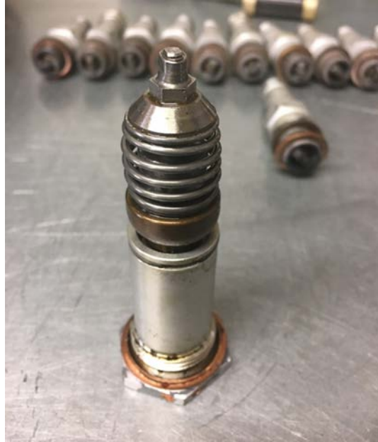
Figure 6. Oil cooler thermostatic bypass valve
