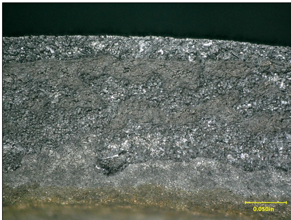
Figure 7. Magnified optical image of the crack fracture surface near the middle of the crack.
