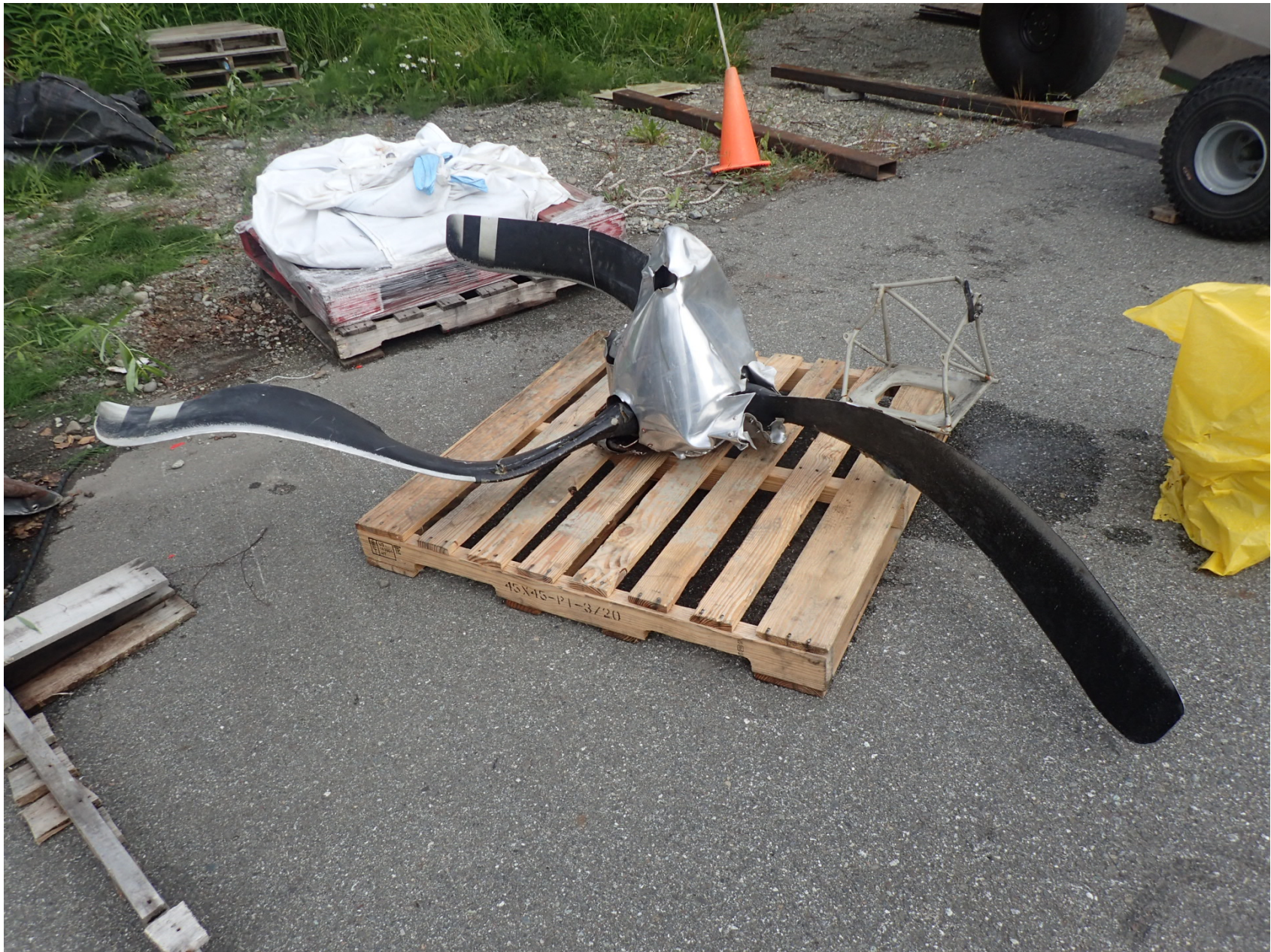
Photo 7 - McCauley model 3GF34C703 propeller indicating blade deformations
