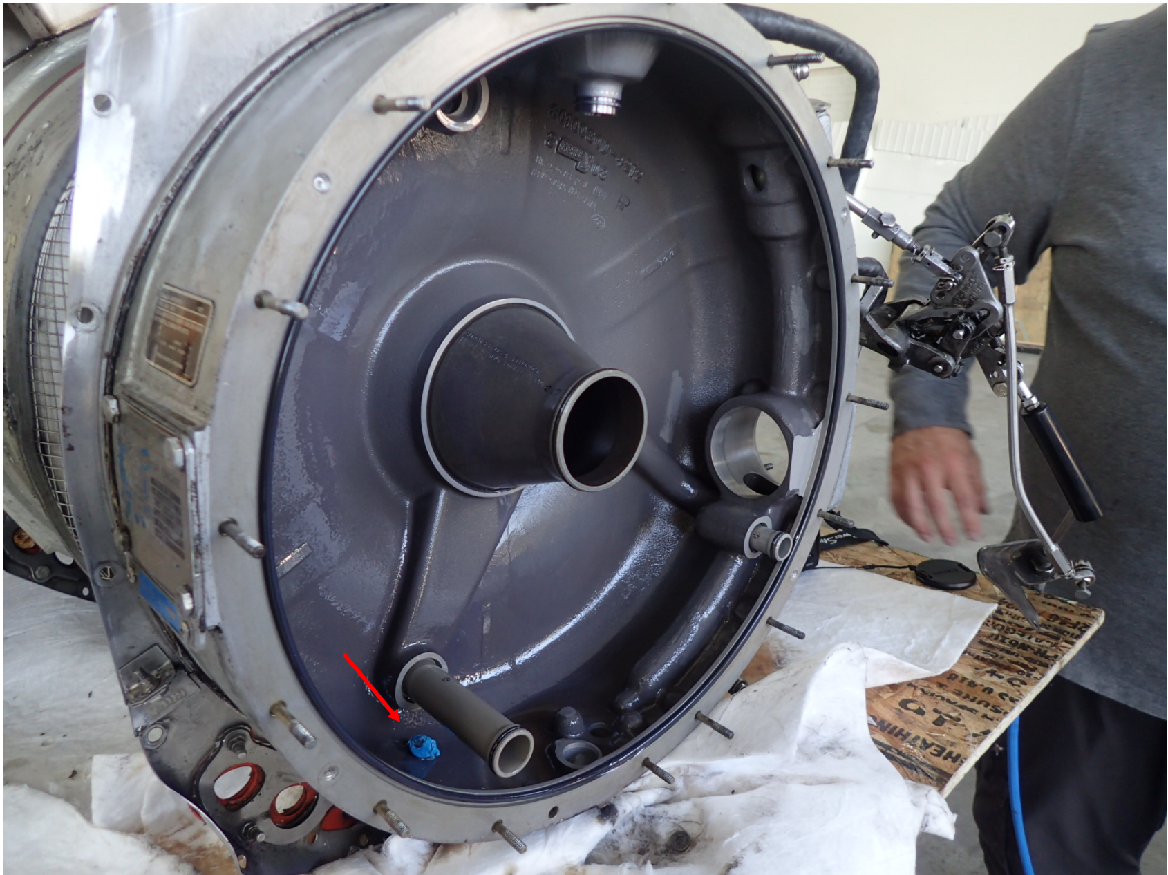
Photo 10 - Engine oil tank with small blue plastic cap evident
