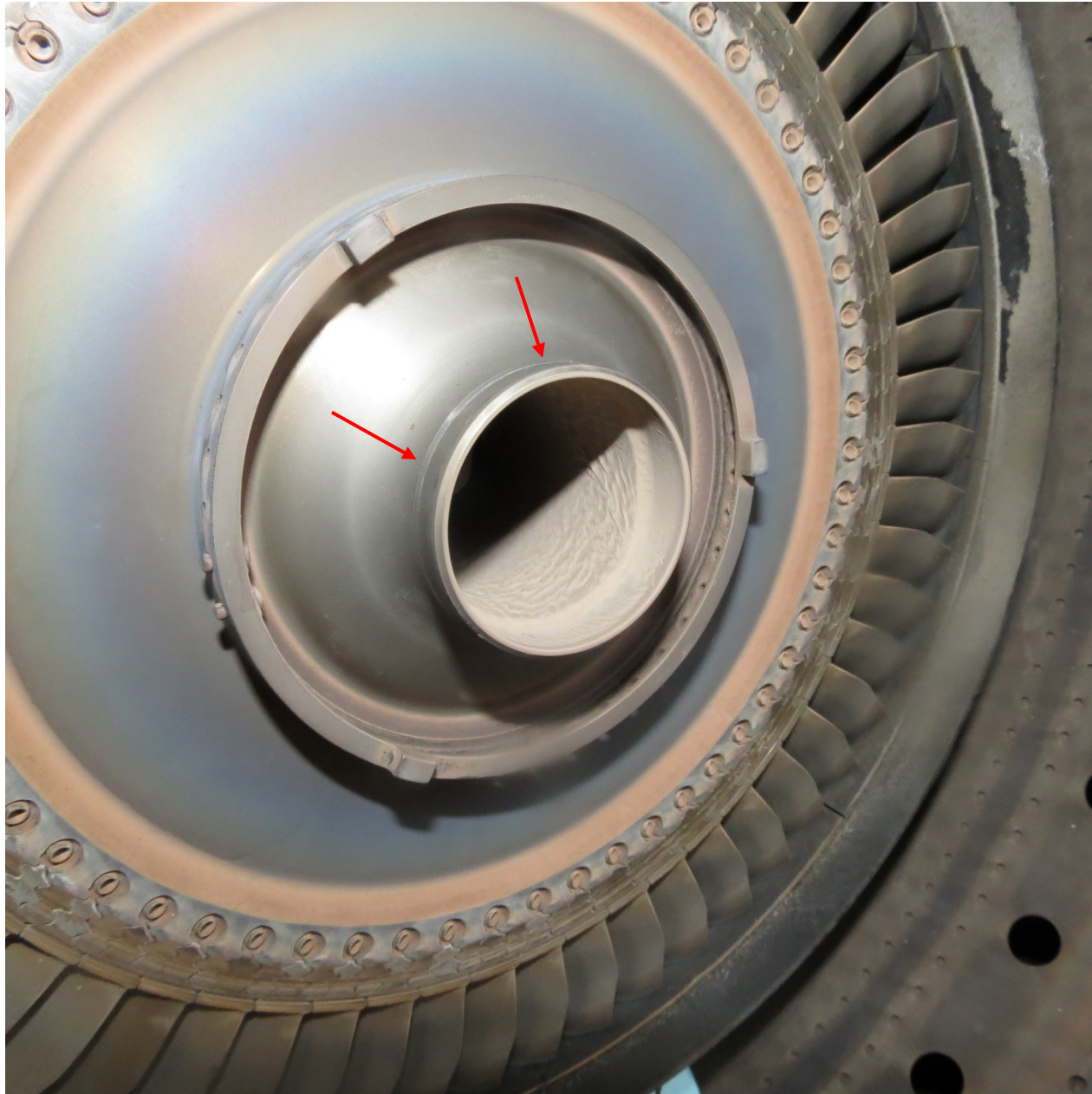
Photo 11 - Engine Compressor turbine (CT) disk bore area with circumferential rubbing marks
