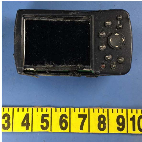
Figure 1. Photo of damaged Garmin GPSMAP 396, as received.
