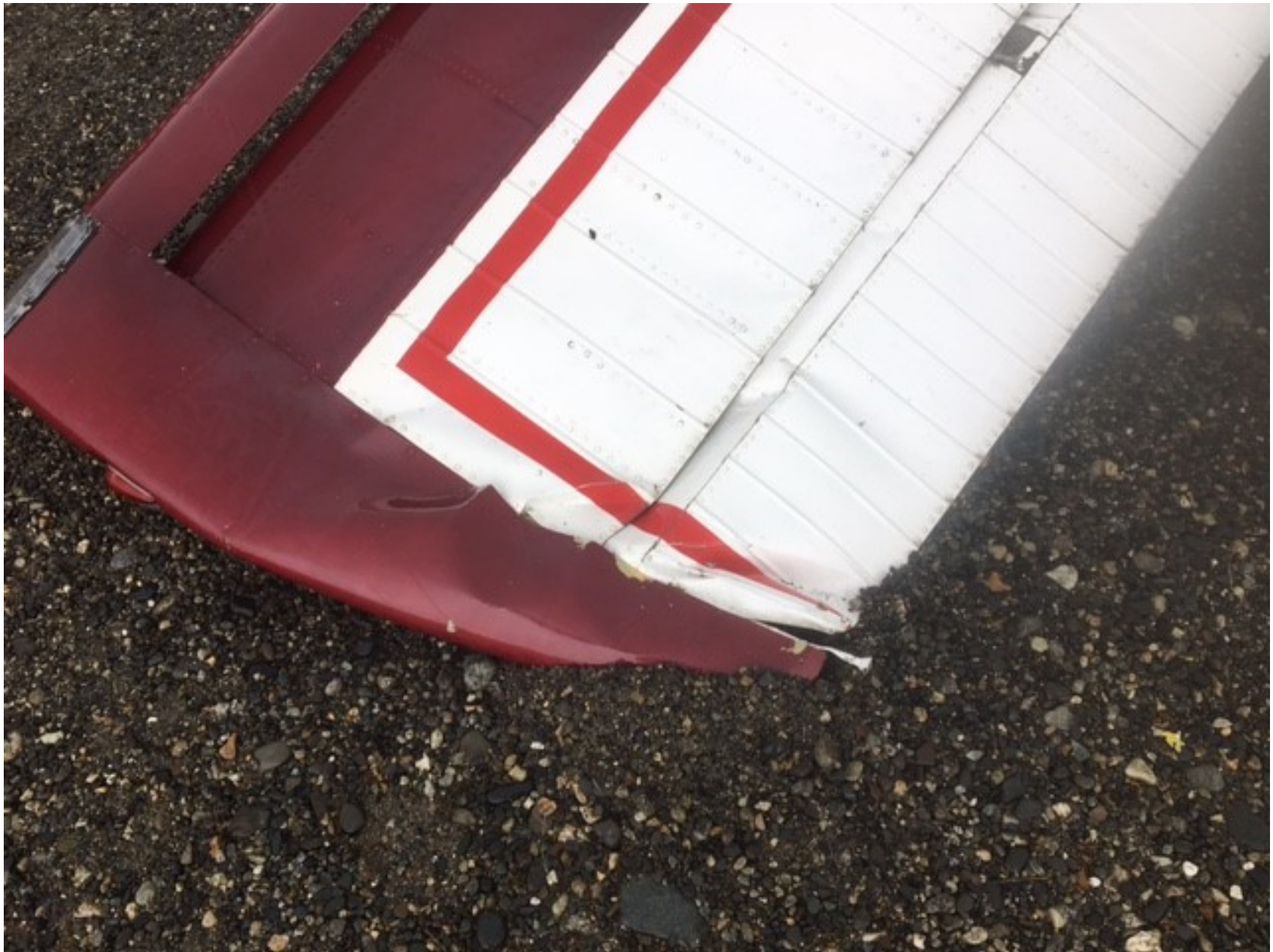
Photo 2 – Left wing and aileron damage
