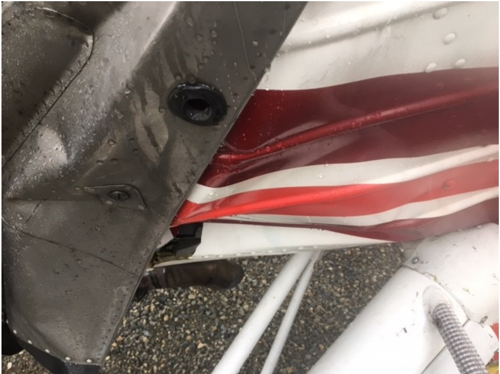
Photo 3 – Left lower fuselage damage
