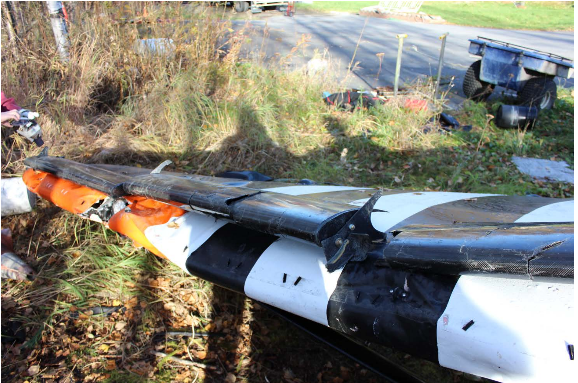
Photo 2 – Right wing's leading-edge slats.
