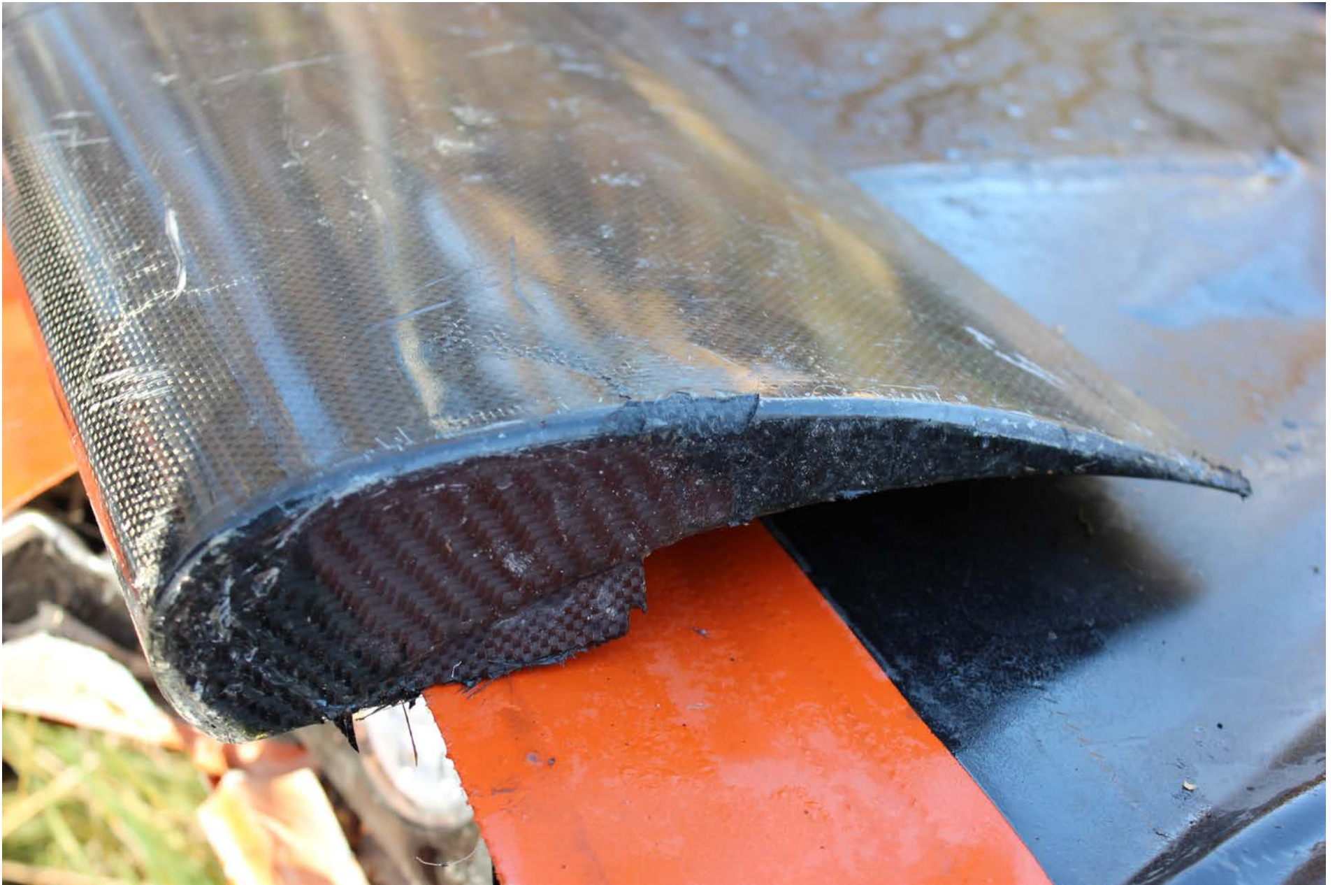
Photo 4 – Right wing leading-edge slat ply bridging.
