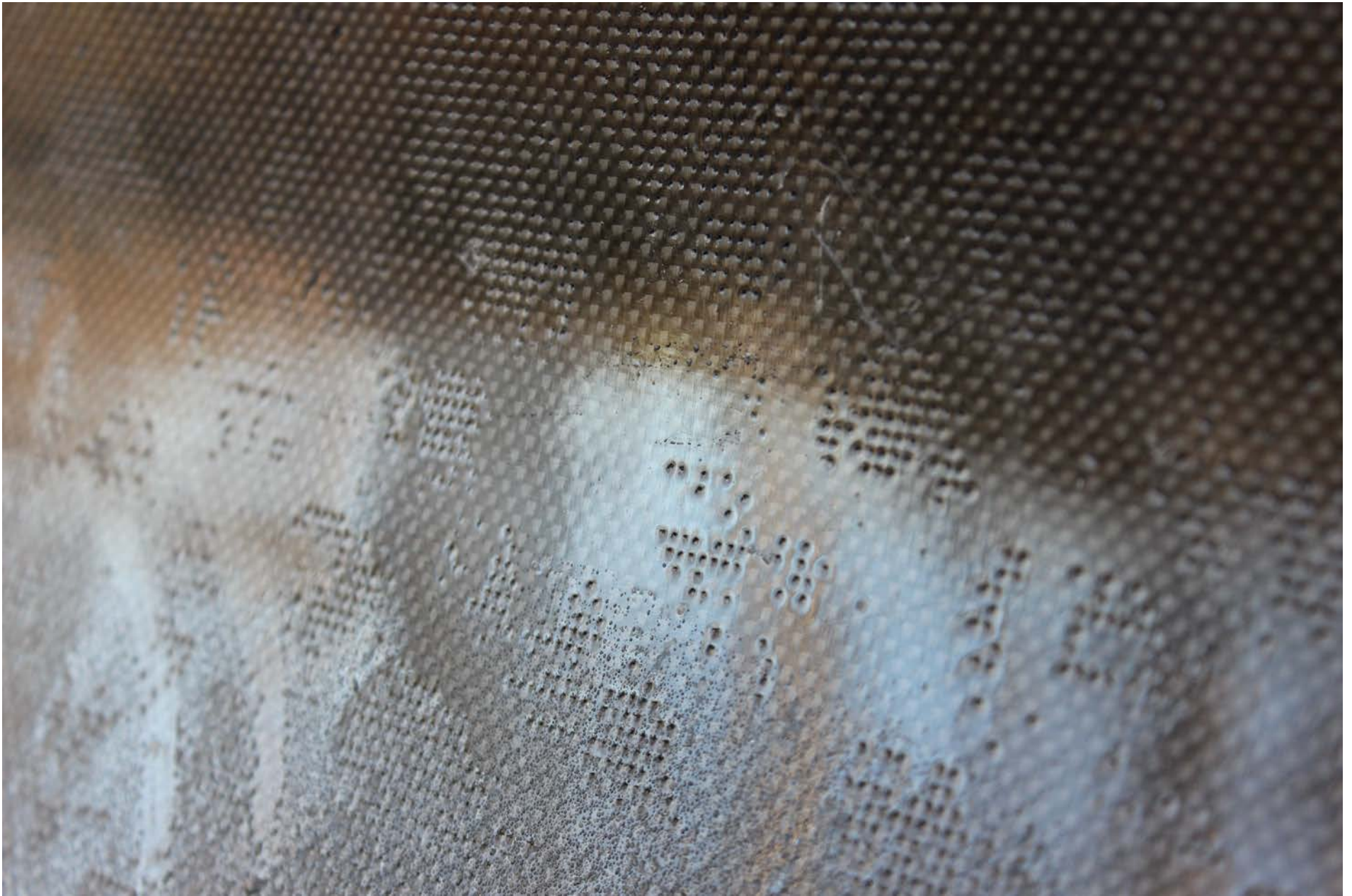
Photo 5 – Left wing leading-edge slat resin starvation.
