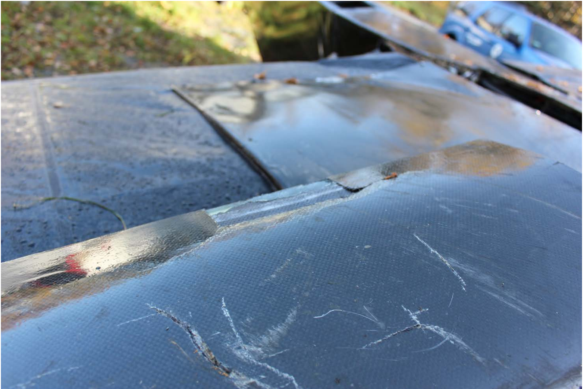
Photo 3 – Right wing leading-edge slat trailing edge bond failure
