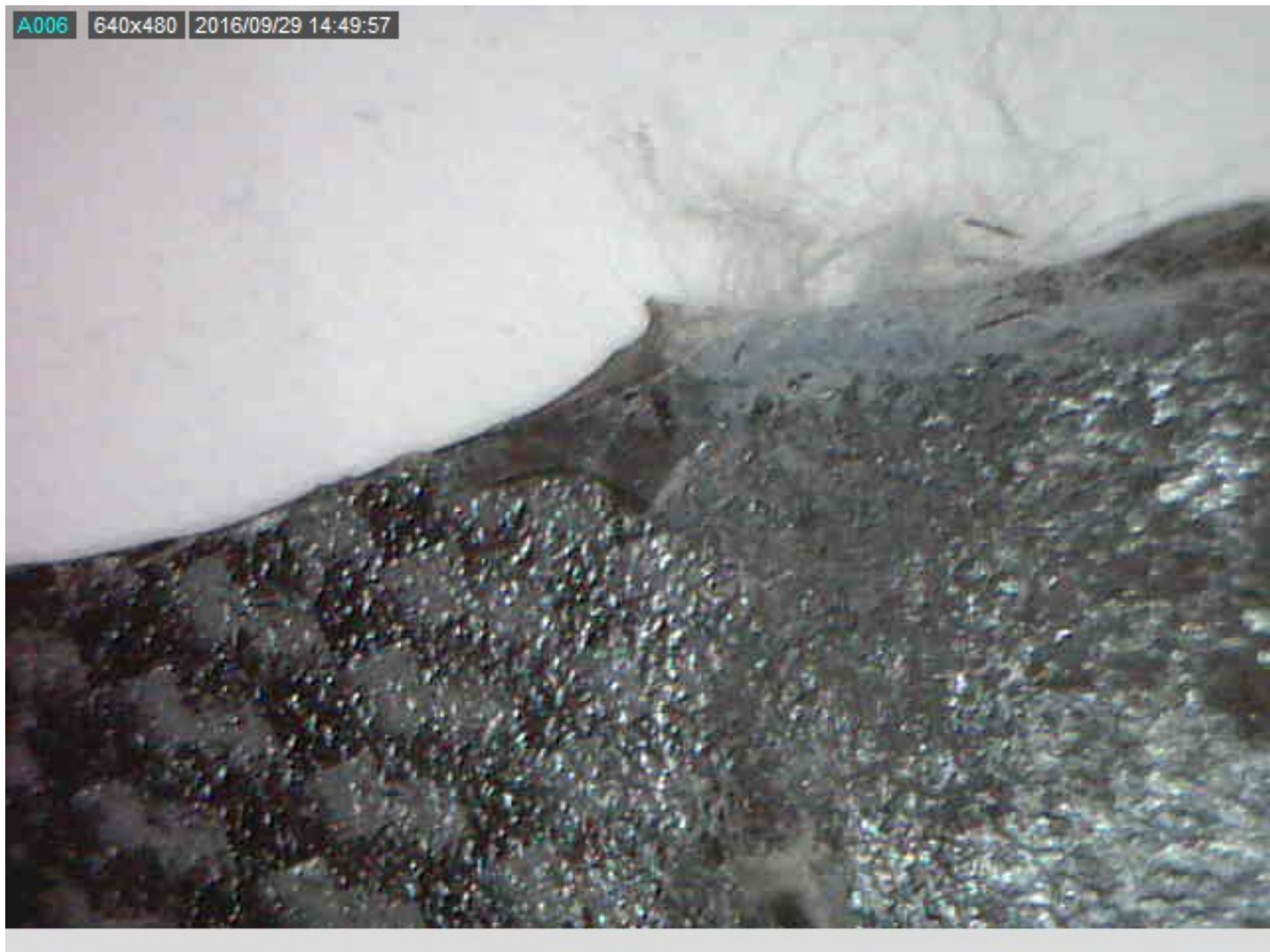
Photo 7 – Microscopic inspection of leading-edge wing slat attachment bracket reveals a lack of adhesion, improper surface preparation and improper adhesive thickness.
