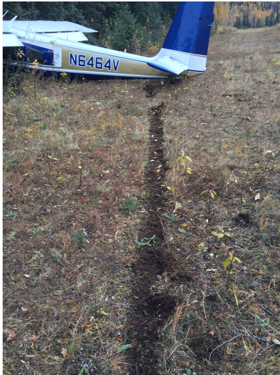
Photo 3 – Trench in airstrip's landing surface.
