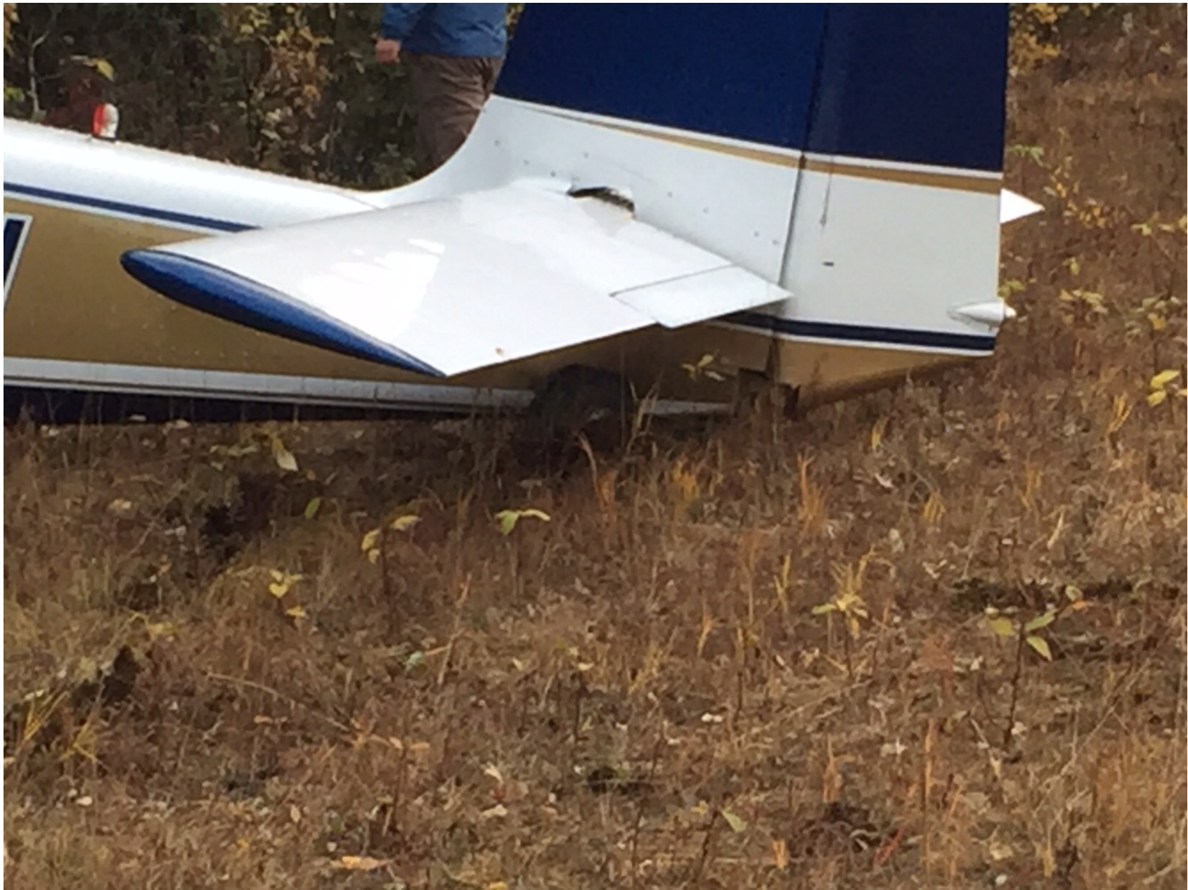
Photo 2 – Tailwheel folded underneath the empennage of the accident airplane at the accident site.
