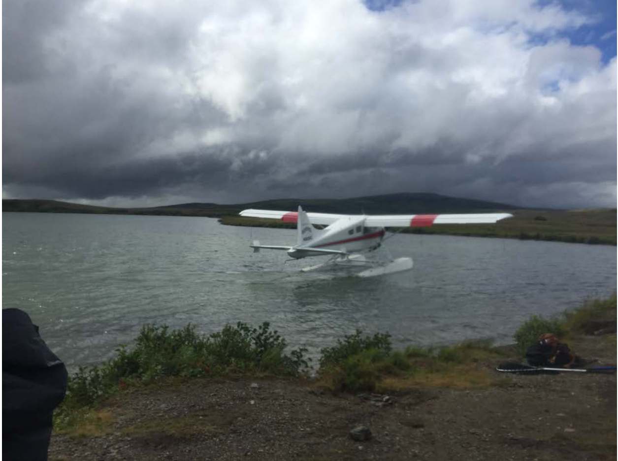
Figure 1 (left side image): The left and right images were taken by the witness. The left image shows the airplane with flaps extended during the taxi prior to takeoff and right image shows the airplane with its flaps retracted during its takeoff run.
