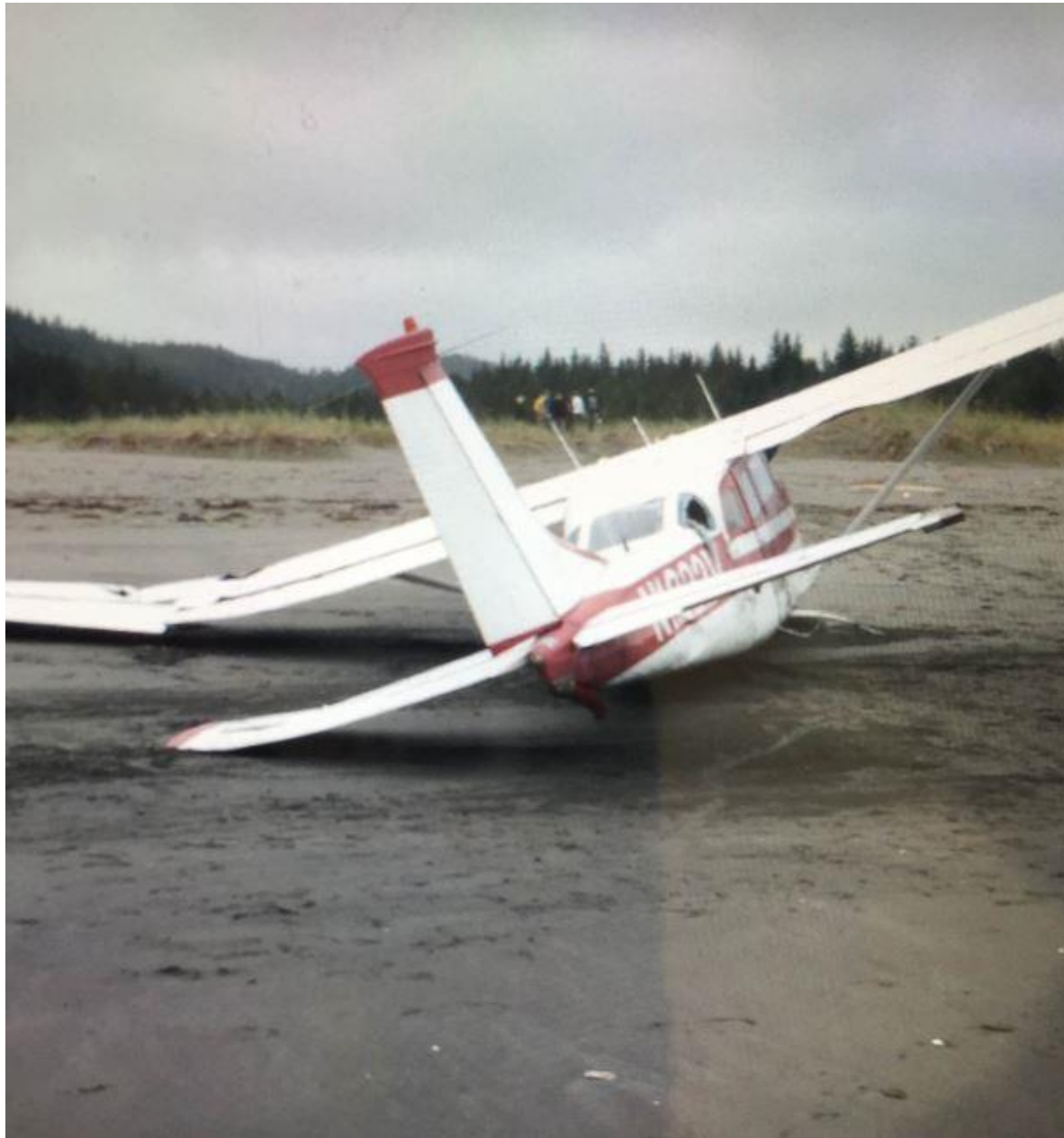
Photo 2 – View of left wing and left horizontal stabilizer (courtesy of the pilot)
