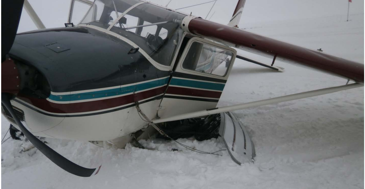
Figure 1: Forward view of the collapsed left main landing gear
