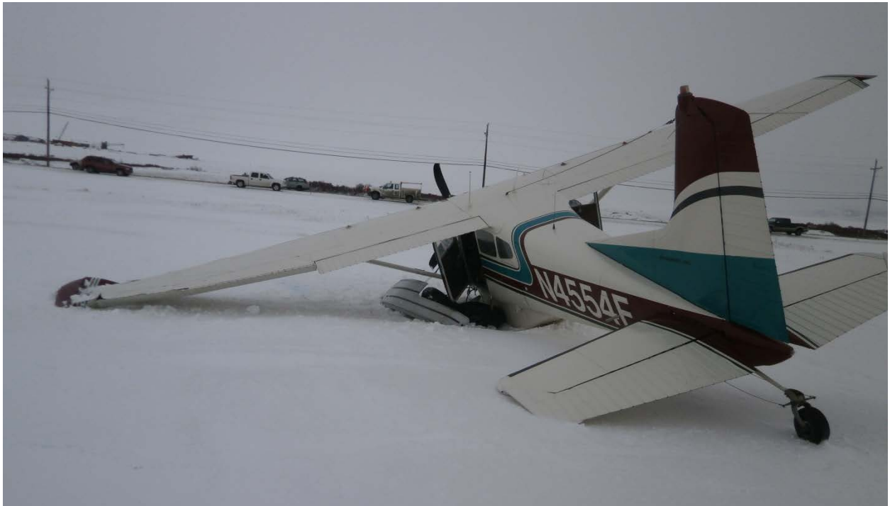
Figure 2: Rear view of the collapsed left main landing gear
