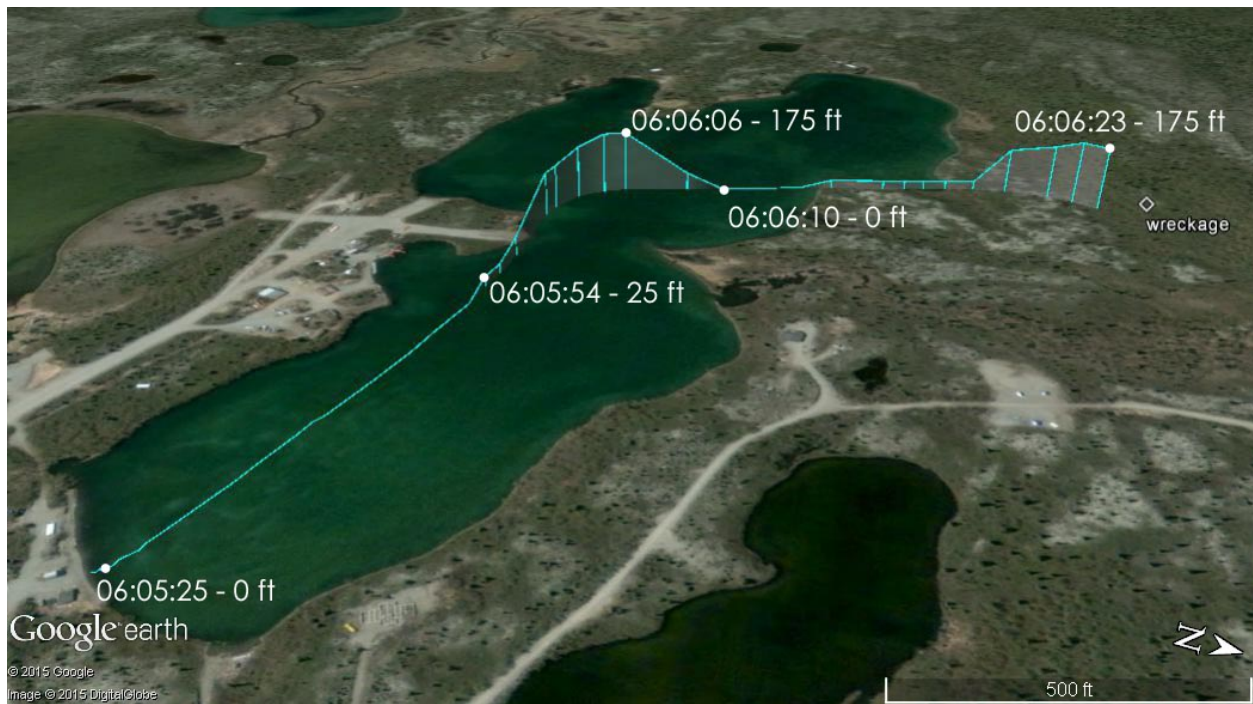
Figure 3. Aircraft path and altitude with selected points.
