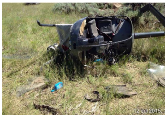
Figure 1. Photograph of substantial damage to Robinson R22 Beta II helicopter
