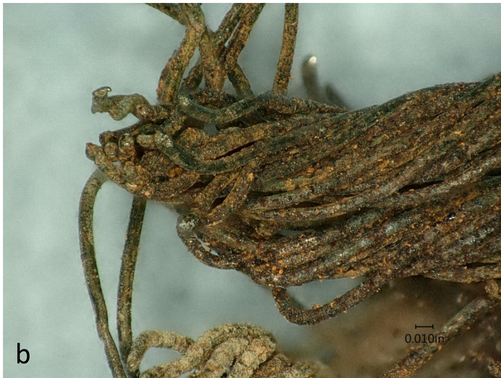
Figure 3 Digital microscope images of the end labeled “wire rope fracture A” in Figure 2 (before cleaning). A higher magnification image is shown in view b.
