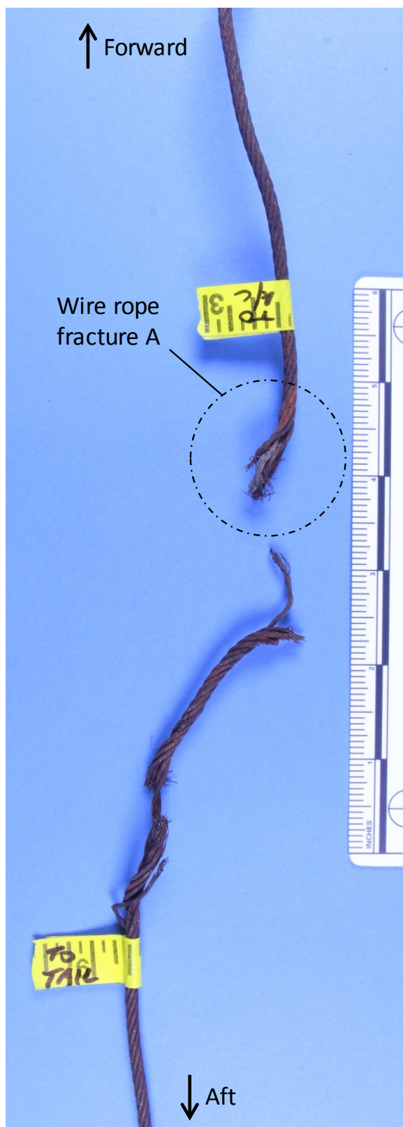
Figure 2 Closer view of the fractured ends on the wire rope pieces.
