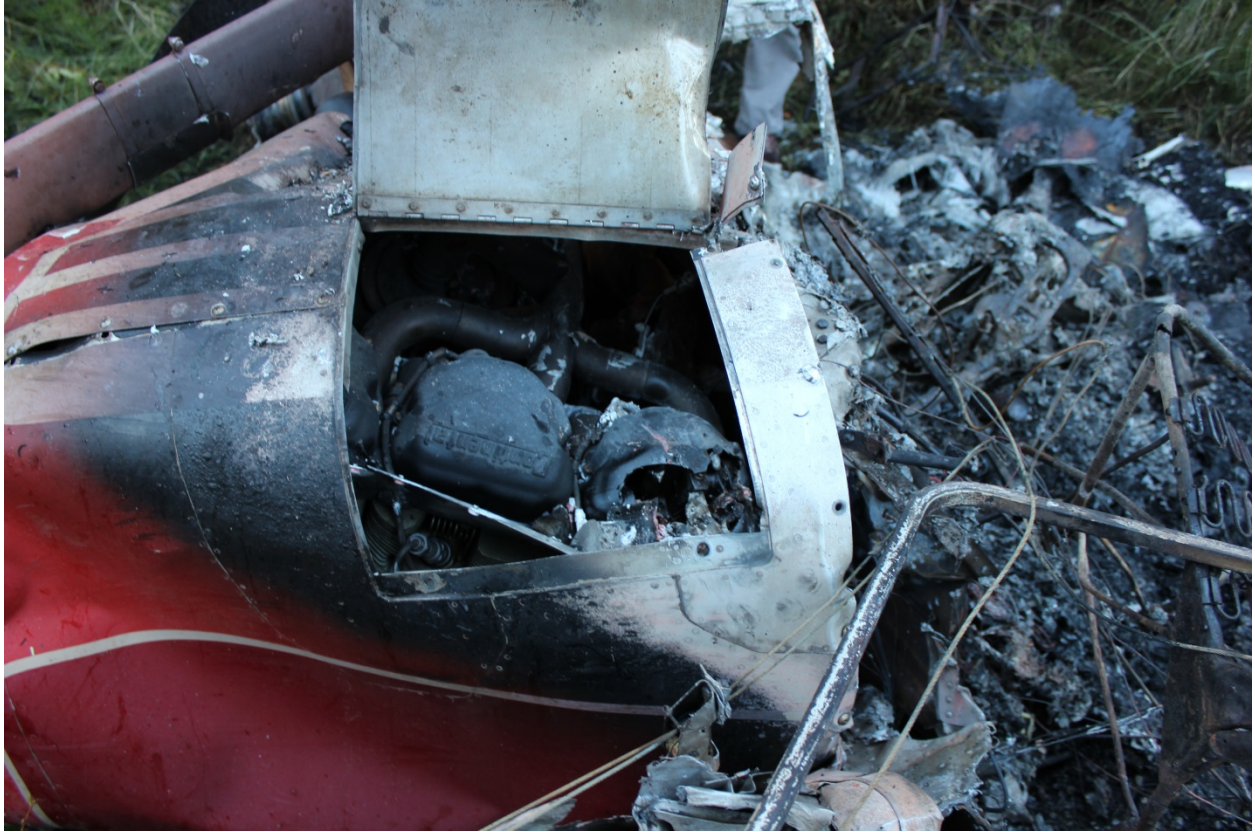
Photo 7: Opened Cowling Access Panel
