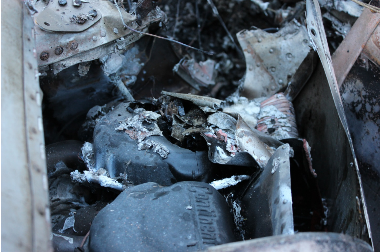
Photo 6: Fractured Rocker Cover
