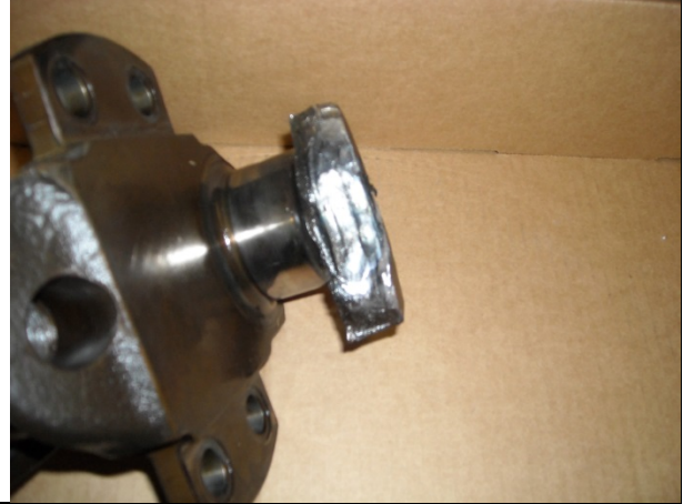
Figure 2. Aft section fracture surface is obliterated
