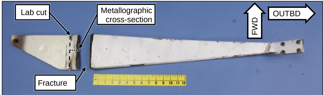
Figure 1. Overall view of the fractured left main landing gear leg showing the lower surface of the leg.
